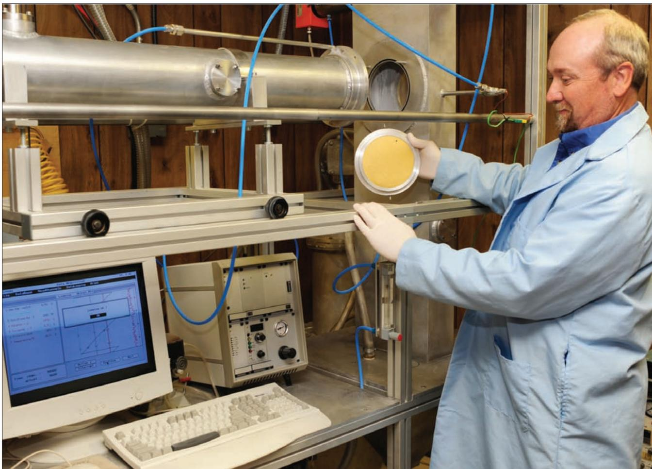
*ETS Laboratory Manager utilizing the filtration performance test apparatus to measure filter media performance under defined conditions to simulate actual baghouse conditions.*
