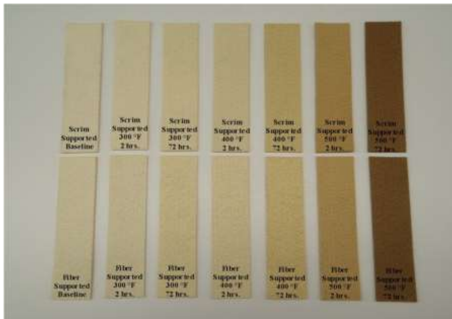
Figure 9: Color Changes Throughout Time vs. Temperature Study of Scrim Supported and Fiber Supported PPS Felt
